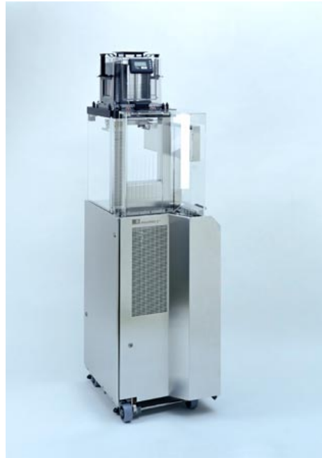
ERGOSPEED II with SMIF pod at ergonomic loading height of 900mm.
