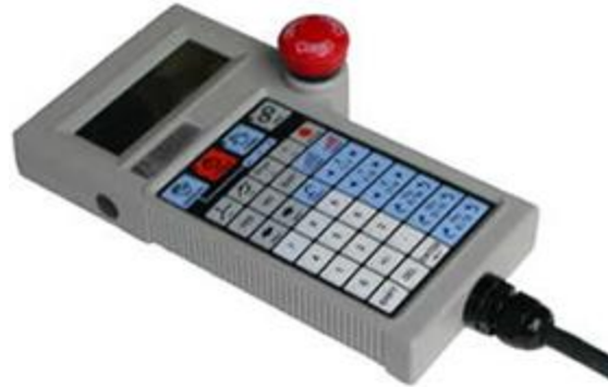
Figure 2-4: Manual Control Pendant
