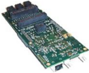
Figure 2-6: Enhanced RIO Module
